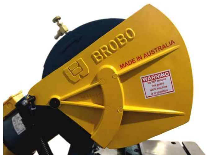
Figure 6. Saw Safety Guard
